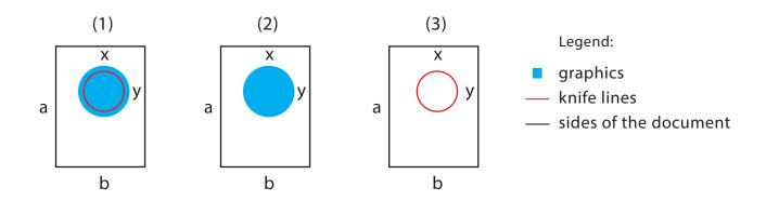
Graphics shall have **3-5 mm bleed** from where the cut is to be made. Printing and other crop marks shall not extend into the bleed area.
